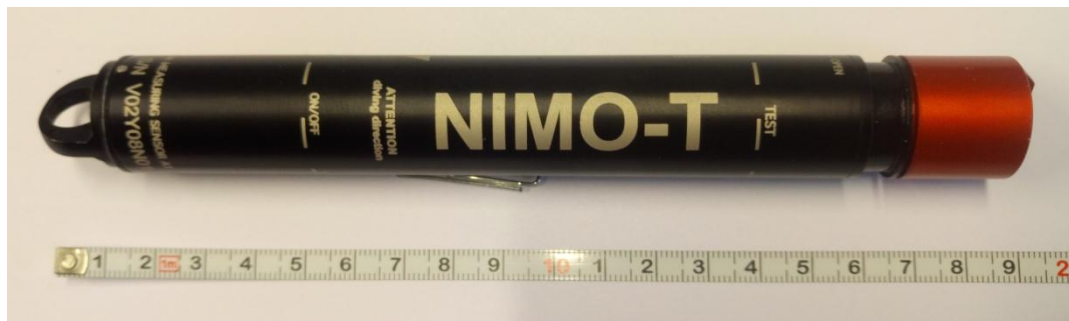
Rys. 1. Non-wired Immersible Measuring Object for Temperature (NIMO-T) logger
